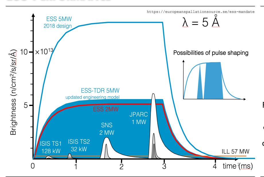
The European Spallation Source (ESS), under construction in Lund, Sweden, will be the most powerful neutron source in the world for neutron scattering experiments. The design of the ESS moderator system to produce both cold and thermal neutrons is based on the concept of a high-brightness bispectral moderator developed at ESS – the so-called quasi-lowdimensional moderators.
