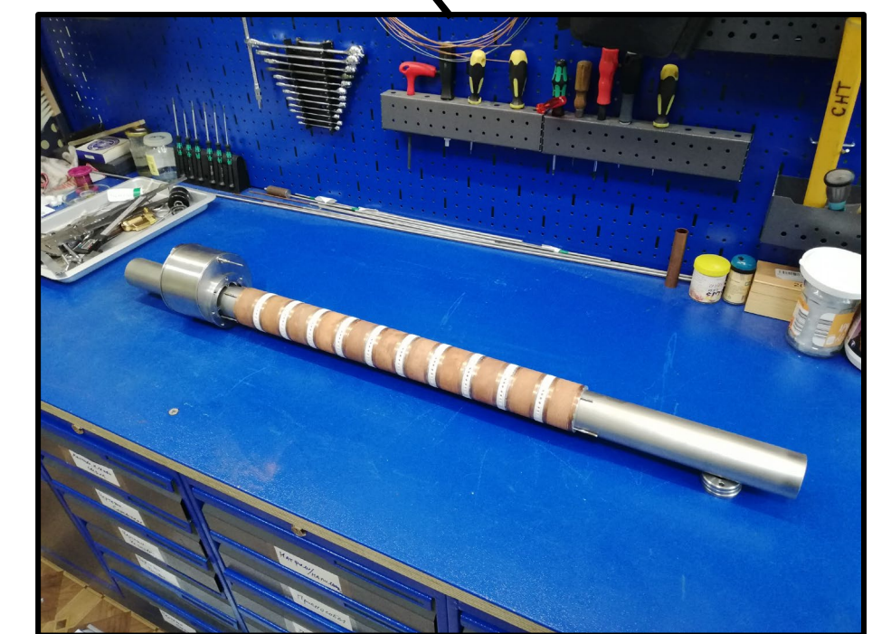
Final (sintered powder) heat exchanger ( T \approx 50 - 350\text{mK} )
