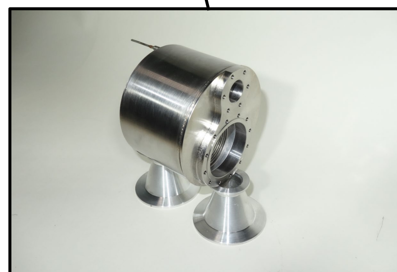
Still (volume with ^3\text{He}/^4\text{He} mixture at T \approx 0.8\text{K} )
