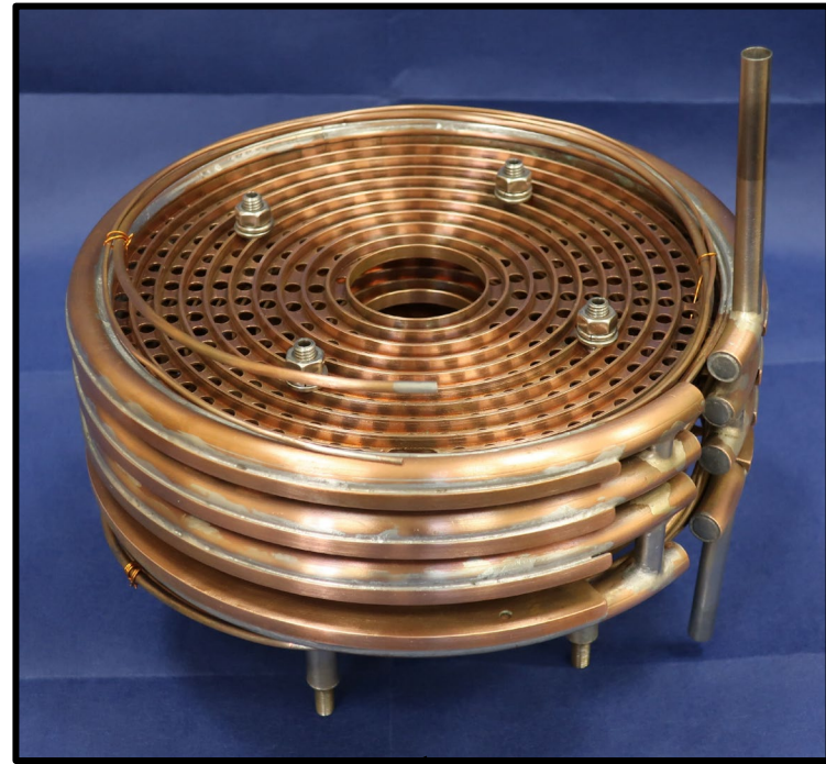
Intermediate heat exchanger ( T \approx 1.5 - 3\text{K} )
