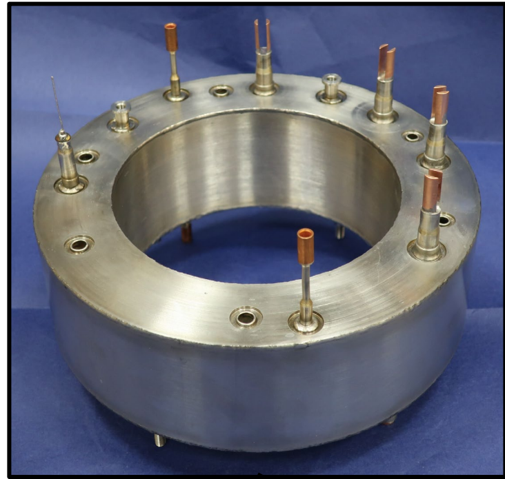
Separator (volume with ^4\text{He} at T \approx 4\text{K} )
