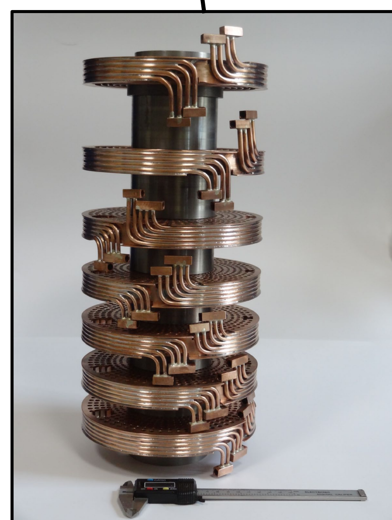
Main (gas) heat exchanger ( T \approx 5 - 250\text{K} )
